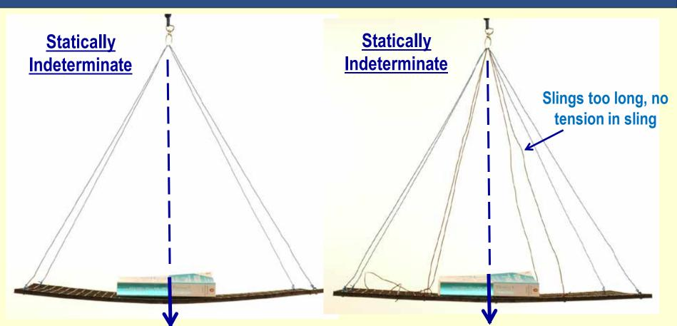
Both rigging schemes are statically indeterminate, need to consider <u>compatibility</u> and <u>equilibrium</u>. Note some slings <u>are not</u> in tension due to sling length misfit in this example. Reduction in module deflection with additional lift points
