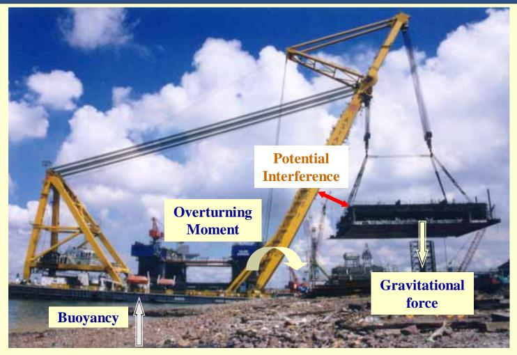
Equilibrium – Buoyancy, gravitational force and overturning moment Compatibility – Geometrically, check potential interference or hook height
