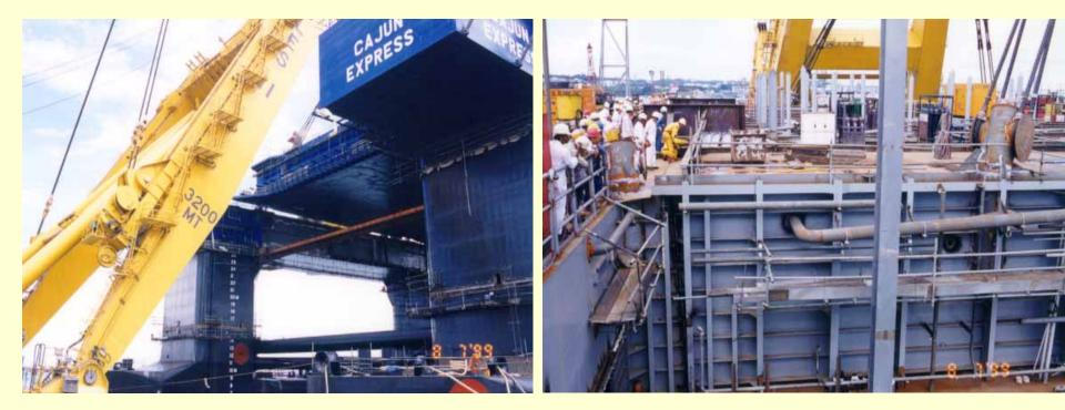
Lowering of centre block in-between the two side blocks Final adjustment for fitting up; note the fabricated trunnion in the fore-ground
