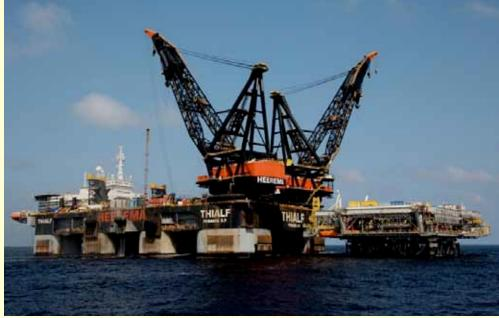
Dual crane-4 lift point lift Statically determinate and sling tensions can be assessed by equilibrium considerations.
