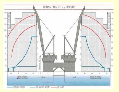
Crane reach-lift capacity curves
