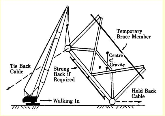
If members during fabrication stage do not have adequate strength, <u>strong back</u> may be needed.
